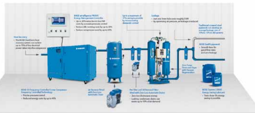
There are a number of areas within a compressed air system where energy savings can be made.
